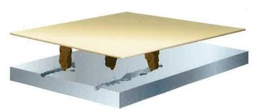
Conventional ceramic abrasive grain is irregular and blocky in shape. Instead of a clean, machining action, the grain tends to "plow" through the metal, causing heat to build up in the workpiece and the abrasive – resulting in a slower cut, shorter belt life and undesirable effects, such as burnishing.
