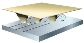
The new precision-shaped grain found in 3M™ Cubitron™ II Belts combines the advanced material properties of our original Cubitron grain with the precise microreplicated structures pioneered in 3M™ Trizact™ Abrasives. As the triangular shaped grain wears, it continuously fractures to form sharp points and edges. The result is a belt that cuts faster, stays cooler and lasts up to 4 times longer than the next best competitive belt.
